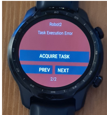
Fig. 1. Photo of the task coordinator app while showing an "urgent" task generated by "Robot2" with the description "Task Execution Error". The second task out of two tasks available in queue for the user is displayed. The "prev" and "next" buttons allows the user to navigate through the tasks queue
