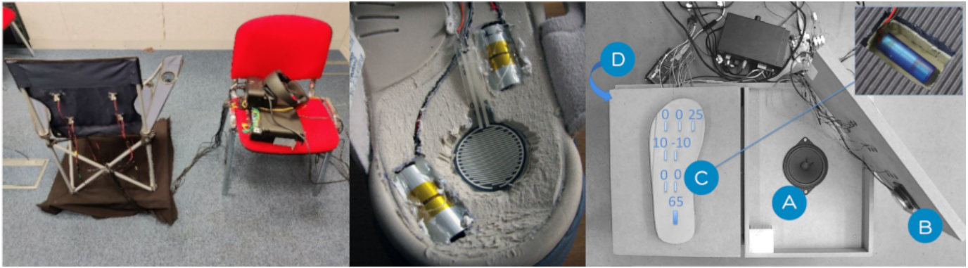
Fig. 3. Haptic motion based on vibrators. Left: Vibrators distributed on the chair enhance the perceived self-motion intensity of a virtual train journey [9]. Middle: an abstract directionless vibration applied at the foot sole can induce directional illusory self-motion [28]. Right: Multi-actuator foot haptics system increases perceived self-motion during VR locomotion [21].
