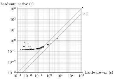
Fig. 4 Comparison of proof times for hardware floating-point arithmetic between vm\_compute and native\_compute. The 4 proofs that fail in both cases appear as a cluster at the top right of the graph.
