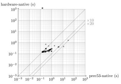
Fig. 5 Comparison of proof times between hardware and 53-bit emulated floating-point arithmetic using native\_compute. The 4 proofs that fail with hardware numbers appear as a cluster at the top of the graph.
