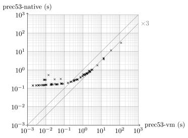
Fig. 3 Comparison of proof times for emulated 53-bit floating-point arithmetic between vm\_compute and native\_compute.
