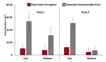
Fig. 5: Experimentaly measured cross sections for the two configurations for each board. Both Silent Data Corruption (SDC) and Detected unrecoverable Errors (DUEs) are shown.
