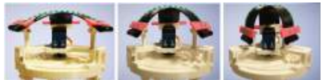
Fig. 4. Soft Y-shaped end-effector. It is composed of a 3D printed Y-shaped strip attached to the moving platform through three joint sliders actuated by the servomotor through a spiral cam. When the spiral cam rotates, the diameter of the circle encompassed by the joint sliders changes, controlling the curvature of the end-effector (in green).
