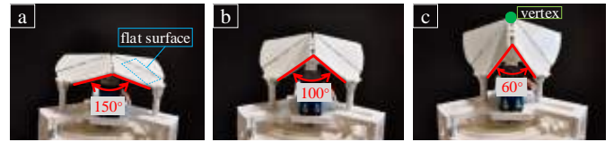
Fig. 6. Origami-inspired rigid end-effector: folding action. The folding of the end-effector is controlled by rotating the spiral cam, which in turn moves the joint sliders towards the center of the platform. Doing so, the end-effector goes from flat ( 150^\circ angle between two adjacent passive panels, left figure) to folded ( 60^\circ angle between two adjacent passive panels, right figure), rendering three edges and one vertex.
