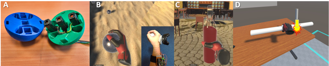
Fig. 1. This paper shows that tangible objects with multiple built-in vibrotactile actuators (A) can effectively render localized vibrotactile cues. These can be used to add spatial information to vibrotactile feedback of interactions with the virtual environment (VE), such as, e.g., feeling textures through a handheld tool (B), feeling contents of a manipulated object (C), or sensing the location of virtual impacts between a virtual handheld object and the VE (D). This opens many perspectives for augmenting passive haptic manipulation in VR.
