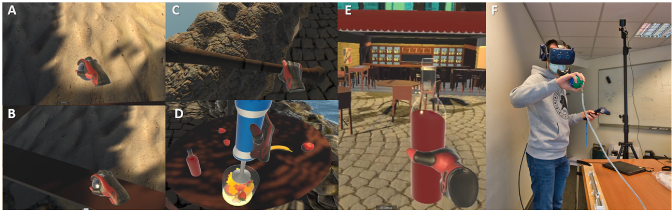
Fig. 9. VR use-case showcasing the different possible interactions. Immersed users can grasp and manipulate objects (F), feel impacts (B,C,D) and textured surfaces through an object held in hand (e.g., sand and wood in A and B), manipulate vibrating tools (the mixer in D) and feel the dynamics of object contents (e.g., wine in the bottle in E). A video of this use-case is available as supplemental material.
