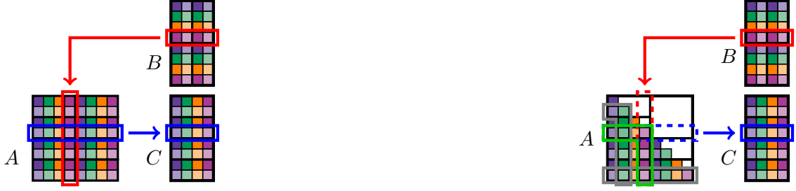
Figure 1: Communications incurred with an A -stationary matrix multiplication, with a 2D BC (2, 4) distribution. Left: storing the whole matrix A . One block of B follows the red path and is sent to p - 1 = 1 nodes. A result computed on a row of A is involved in a reduction operation on q nodes (blue path), resulting in q - 1 = 3 messages sent. Right: storing the lower half of A . Both types of communication now involve p + q - 1 = 5 nodes, resulting in 4 messages sent. Parts of the matrix where fewer nodes are involved are highlighted in grey.
