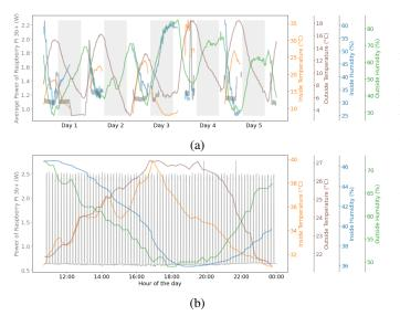
Fig. 2: (a) The in-hive temperature and humidity, the external temperature and humidity, and the averaged Raspberry Pi 3b+ consumption during one week of Spring 2022 in Cachan (France). (b) The in-hive temperature and humidity, the external temperature and humidity, and the Raspberry Pi 3b+ consumption showing consecutive wake-ups during 13 hours of one day in Summer 2022 in Cachan (France).
