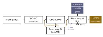
Fig. 1: Architecture of the deployed system showing essential hardware, energy node, and network
