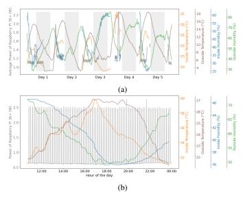
Fig. 2: (a) The in-hive temperature and humidity, the external temperature and humidity, and the averaged Raspberry Pi 3b+consumption during one week of Spring 2022 in Cachan (France). (b) The in-hive temperature and humidity, the external temperature and humidity, and the Raspberry Pi 3b+consumption showing consecutive wake-ups during 13 hours of one day in Summer 2022 in Cachan (France).
