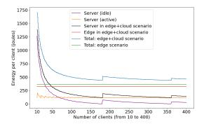
Fig. 6: Simulation of energy consumption for all entities in a client-server scenario with no loss. Number of clients allowed in parallel in time slots: 10.
