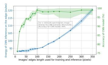
Fig. 5: Energy of CNN model execution and its accuracy on the test set as a function of training set's images' size.
