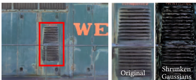
Fig. 3. We visualize the 3D Gaussians after optimization by shrinking them 60% (far right). This clearly shows the anisotropic shapes of the 3D Gaussians that compactly represent complex geometry after optimization. Left the actual rendered image.
