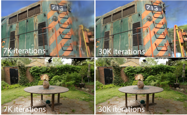
Fig. 6. For some scenes (above) we can see that even at 7K iterations (~5min for this scene), our method has captured the train quite well. At 30K iterations (~35min) the background artifacts have been reduced significantly. For other scenes (below), the difference is barely visible; 7K iterations (~8min) is already very high quality.
