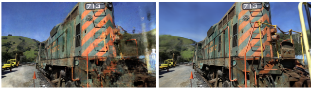
Fig. 11. Comparison of failure artifacts: Mip-NeRF360 has “floaters” and grainy appearance (left, foreground), while our method produces coarse, anisotropic Gaussians resulting in low-detail visuals (right, background). TRAIN scene.
