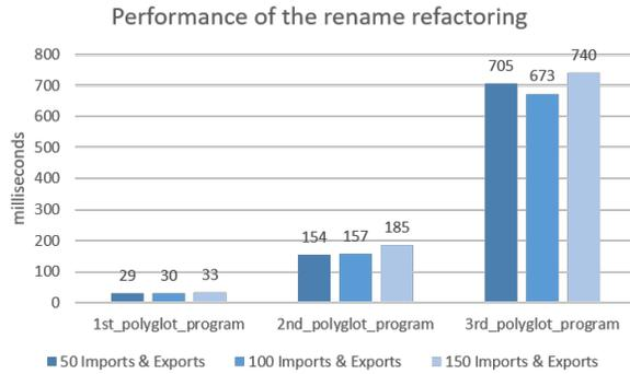
Fig. 8. Performance of the rename refactoring polyglot service.
