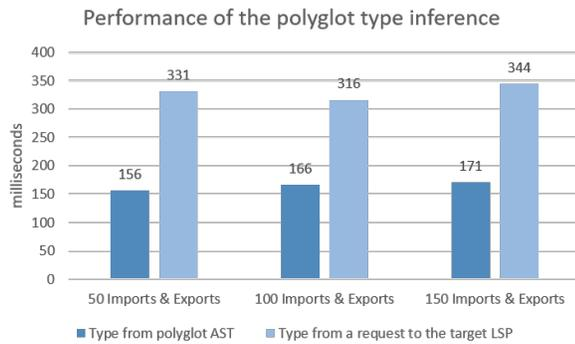
Fig. 9. Performance of the type inference polyglot service.
