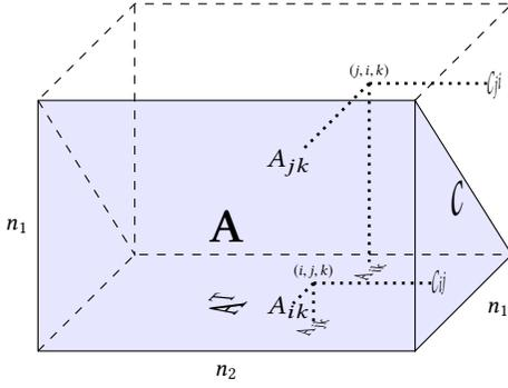
**Figure 1: Iteration space of SYRK with a total of  $n_1 n_2 (n_1 + 1)/2$  iteration points. Iteration  $(i, j, k)$  and its projections are shown along with its symmetric partner  $(j, i, k)$  as described in Lemma 3.**
