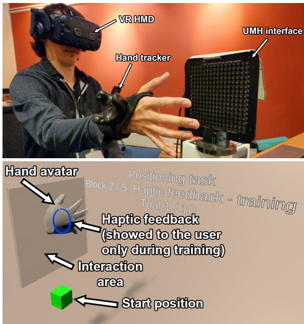
Fig. 2. (Top) Experimental setup. Participants seat near the ultrasound haptic interface, with their dominant hand facing the device. They wear a VR HMD and a tracker. They hold a controller in their other hand to validate trials and start blocks. (Bottom) VR scene, where the interaction area is indicated by a translucent squared area. During training only, the scene also showed the rendered haptic sensations (blue circle in this case).
