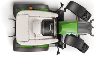
Fig. 12. The slender design that characterizes this tractor, “Fendt 200 Vario”, allows it reaching in this case up to 52°-steering angle with the original-equipment wheels [26].
