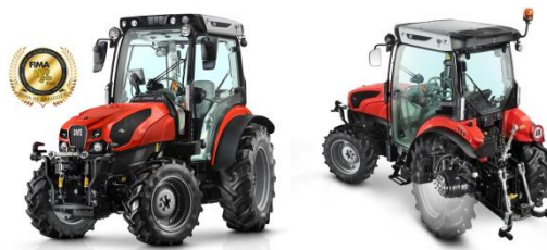
Fig. 13. The “SAME Frutteto CVT Activesteer” has a rear wheel steering angle of 18° [27].
