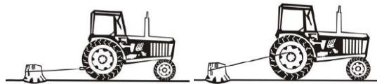
Fig. 10. (left) an example of safe hitching; (right) an example of unsafe hitching [25].
