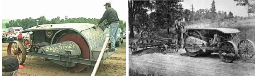
Fig. 15. 1WD farm tractor “Gray 18-36” (1916); it uses a unique rear drum-drive system [29].
