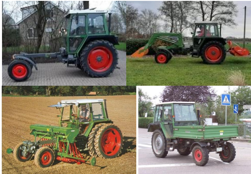
Fig. 22. 32.9-kW 2WD implement carrier “Fendt F 345 GT” (1984) as it is (top left) or with a front loader and a rear rotary harrow (top right), a front seed drill implement (bottom left) or a dumper loading bay (bottom right) [37, 38].
