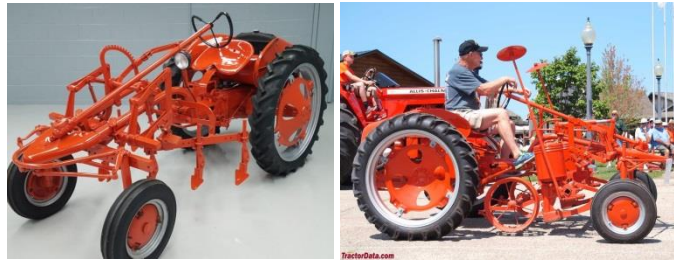
Fig. 20. 2WD implement carrier “ Allis-Chalmers G ” (1948) (left) equipped with a cultivator [35] or (right) equipped with a mechanical seed drill [36].
