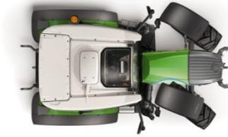
Fig. 12. The slender design that characterizes this tractor, “Fendt 200 Vario”, allows it reaching in this case up to 52^\circ -steering angle with the original-equipment wheels [26].
