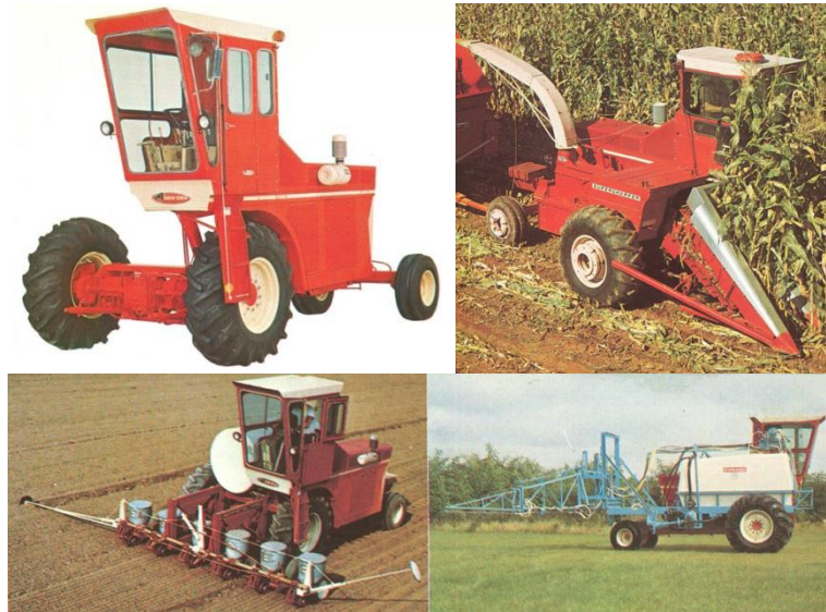
Fig. 26. 2WD universal operating machine “AVCO New Idea Uni-System 700” (1980) as it is (top left), with a forage harvester equipment (top right), with a seed drill system (bottom left), with a boom sprayer equipment (bottom right).
