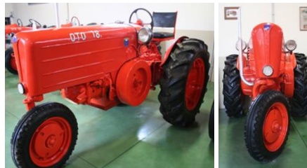
Fig. 16. 2WD farm tractor “OTO R3” (1950) (pictures taken from [30]); no differential is present on the rear wheels, the steering manoeuvres were performed acting at the same time on the steering wheel and on pedals controlling some clutches and the brakes.
