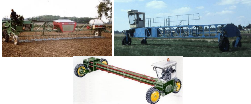
Fig. 25. Universal operating machine “Gantry”; first 2WD prototype by Dowler (1970) equipped as fertilizer spreader (top left); first 2WD commercial version “Monotrail” (1983) as it is i.e., without any implement installed (top right); latest 4WD 12-m-width version (1990) as it is [46] (bottom).
