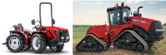
Fig. 5. (left) 4WD special-purpose articulated tractor “Antonio Carraro SN 5800 V” [14], (right) 4WD universal articulated tractor “Case IH Steiger 540” equipped with half-tracks instead of the pneumatic wheels [15].
