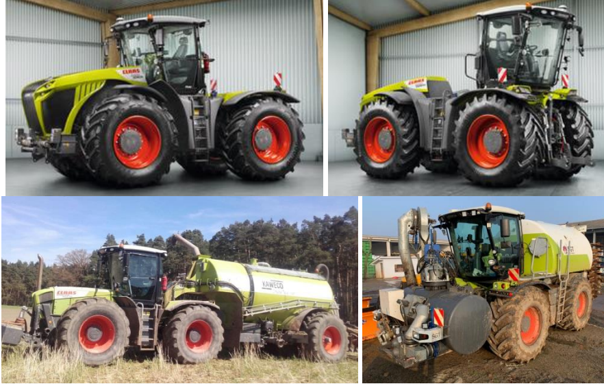
Fig. 24. 4WD 4-wheel-steering multi-purpose tractor with rotating central cab “Claas Xerion Trac VC” (2005) in the standard configuration (top left), with the cabin in the reverse position (top right), with a specific trailed (bottom left) or mounted (bottom right) manure spreader equipment [43].
