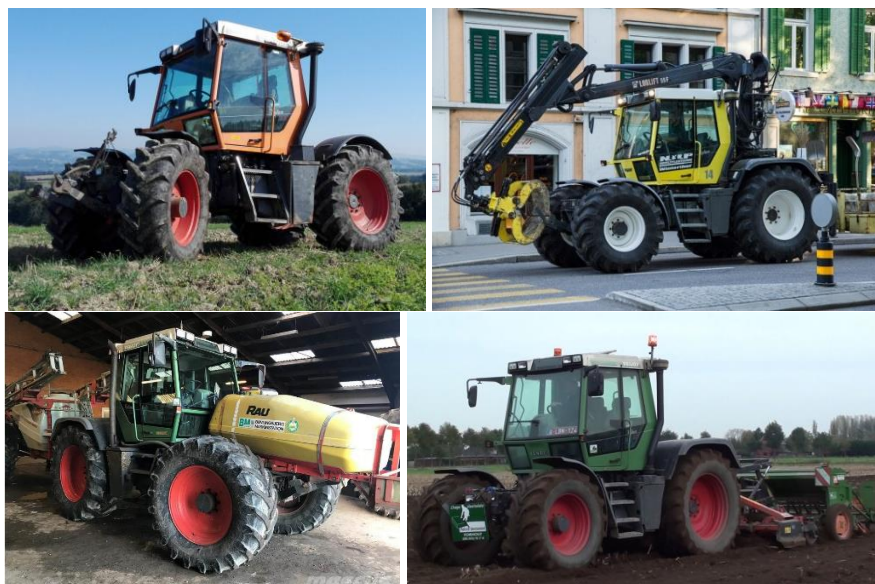
Fig. 23. 4WD multi-purpose tractor with central cab “Fendt Xylon 320” (1994) as it is (top left) or with a plier (top right), a boom sprayer equipment (bottom left) or a sowing implement (bottom right) [39–42].
