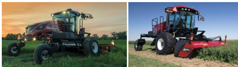
Fig. 28. 2WD windrower with reversible driving commands and two pivoting wheels “MacDon M150” (2001) [47].
