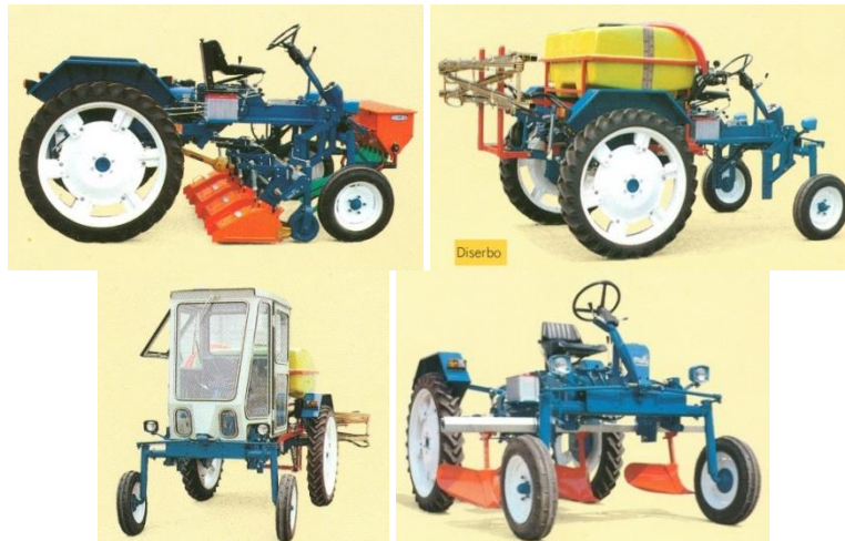
Fig. 21. 2WD implement carrier “ FM Multi 28 L – 33 L ” (precise year unknown) with different accessories/implements: seed drill (top left), boom sprayer (top right), cabin (bottom left), ridger plough (bottom right).
