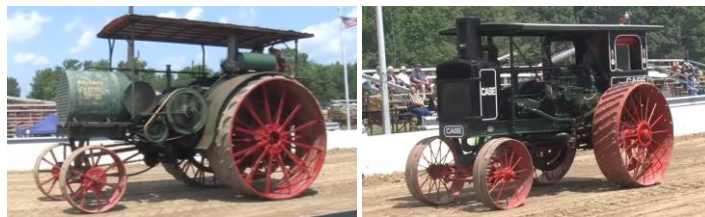
Fig. 2. (left) 2WD gasoline-fuelled farm tractor “Aultman-Taylor 30-60” (1911); (right) 2WD kerosene-fuelled farm tractor “Case 20-40” (1919) [10].
