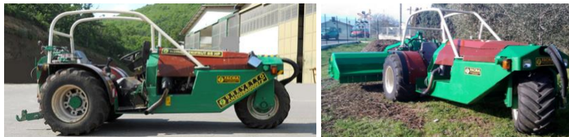
Fig. 18. 3WD hydrostatic farm tractor “Fagma Trifrut” (2010) (left) as it is or (right) with a rear hoeing machine [31, 32].
