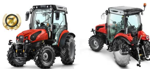
Fig. 13. The “SAME Frutteto CVT Activesteer” has a rear wheel steering angle of 18^\circ [27].
