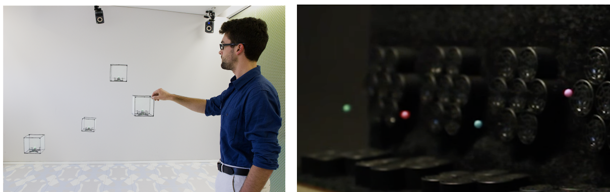
Figure 7 – Recent research prototypes that can position physical objects in three-dimensional space. BitDrones (left image) uses rotors, while the Floating Charts device (right image) uses acoustic levitation. Sources: BitDrones http://www.humanmedialab.org/blog/bitdrones (2015). Credit Calvin Rubens, Sean Braley, Antonio Gomes, Daniel Goc, Xujing Zhang, Juan-Pablo Carrascal, and Roel Vertegaal. Floating Charts https://www.youtube.com/watch?v=3-Tjcz16rXU (2016). Credit Themis Omirou, Asier Marzo Perez, Sriram Subramanian, and Anne Roudaut. Permissions pending.
