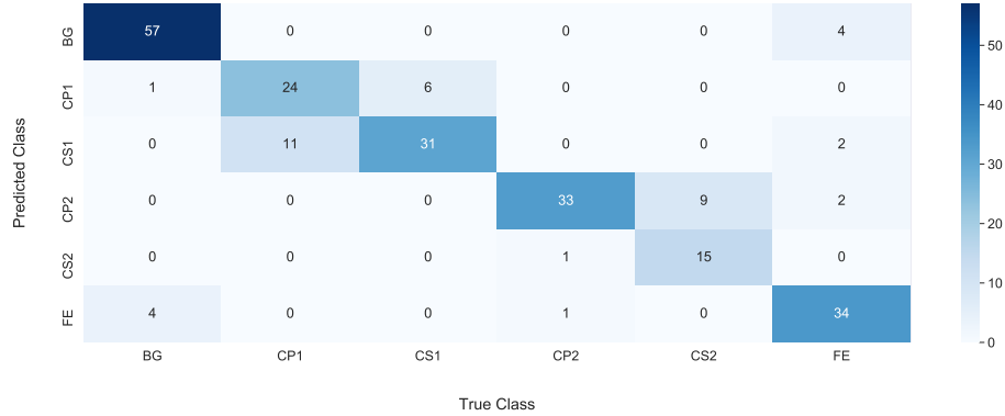
Fig. 4. Confusion matrix for the evaluation of the 235 test data samples using the best performing log-STFT multimodal network architecture.
