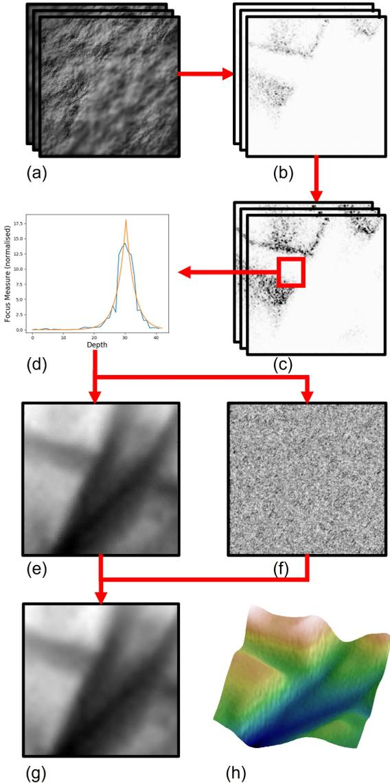
**Fig. 1** Our depth from focus pipeline. Starting from the acquired focal stack  $\mathcal{I}$  (a), we compute a Focus Measure map  $\mathcal{F}$  (b) and a low-pass version  $\tilde{\mathcal{F}}$  (c) through Gaussian smoothing. For each pixel, we perform our Peak Estimation procedure (d), yielding a depth map  $\mathcal{D}$  (e) and a reliability map  $\mathcal{R}$  (f). Finally, we apply an adaptive MLS filter from these two maps to obtain our final depth map (g) giving a 3D profile (h).
