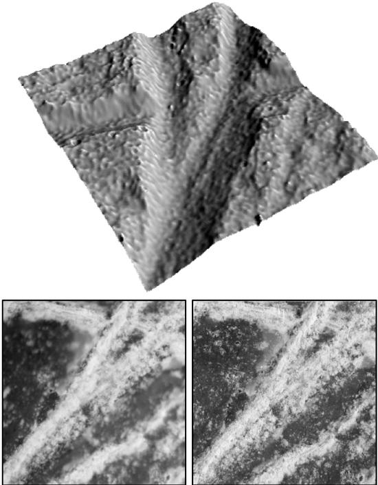
**Fig. 10** Results get on a real-word stack from an engraved stone. Top: 3D profile of the acquired engraving area. Bottom left: blurry image obtained on the image stack. Bottom right: reconstituted clear image of the engraving.
