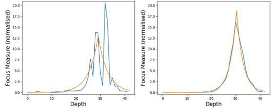
**Fig. 2** Demonstration of the importance of the Gaussian filter. Left: curve of FM of one pixel as a function of depth  $z$ , on an FM where the Gaussian filter is not applied. Right: curve of FM of the same pixel as a function of depth  $z$ , on an FM where the Gaussian filter has a width of 20.
