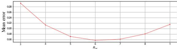
**Fig. 5** Average absolute error over 20 synthetic stacks as a function of the window size  $n_w$ .
