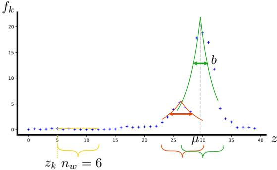
**Fig. 3** Illustration of our sliding window strategy. The FM profile is shown as blue crosses and three position of the window are depicted in yellow, red, and green respectively. The window size  $n_w$  is constant, and each window starts at a position  $z_k$ .
