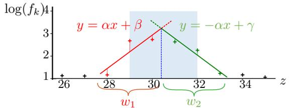
**Fig. 4** Illustration of the *Triangle* method. In log space, the current window  $[28, 31]$  is partitioned within two parts. Each part is approximated by a piece-wise linear function having opposite slopes.
