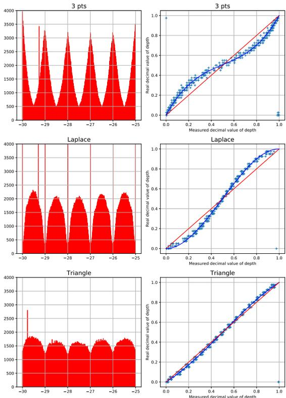
**Fig. 9** For each of the three methods, the left histograms show the distributions of the computed depth values for the 80 depth maps  $\mathcal{D}$ , and the right scatter plots show the ground truth decimal depth values as a function of the decimal of the computed depth values. Those plots also include least-squares cubic approximations of this function (blue curve), and the ideal identity relation in red.
