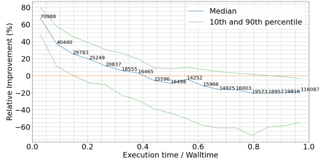
(b) Evolution of response time for jobs as a function of the ratio t^{real}/t^{estimate}
