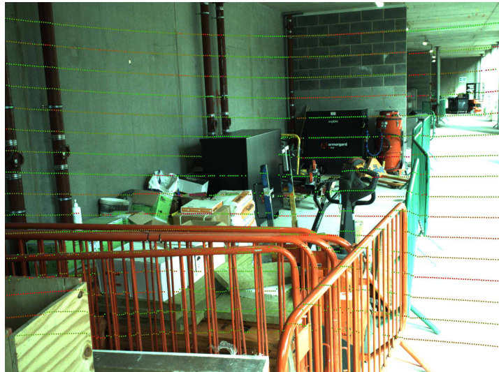
Fig. 6. Example of projecting of LiDAR points onto the corresponding image
