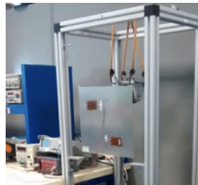
Figure 3: Ampere's vibrating rig [Zieliński 2015]
