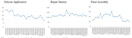
Fig. 1. Number of defects per unit found at different stations.
