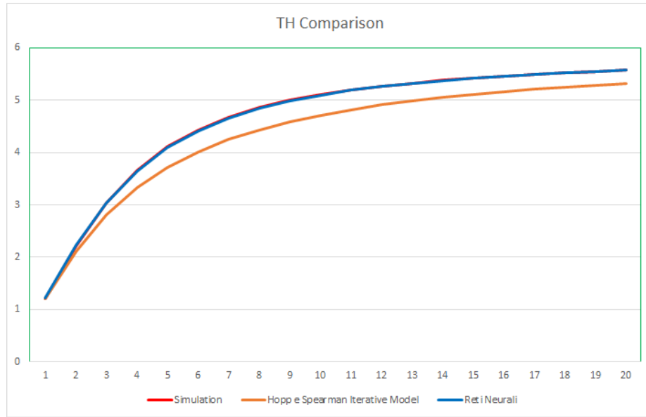
Fig. 5. Comparison of the proposed deep learning neural network model with the iterative Spearman et al. [8] model and the data from the simulation tool in a scenario with \alpha = 3 .
