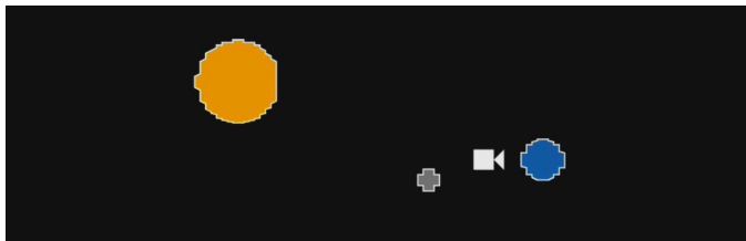
Fig. 4: A schematic overview of floating point precision error when rendering small objects at large distances from the coordinate system origin in camera space. In this image, 5 significant mantissa bits are used, the coordinate system origin is the center of the orange sphere. Catastrophic cancellation causes objects close to the camera (blue and grey spheres) to suffer from floating point aliasing.
