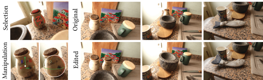
Fig. 1. NeRFshop enables intuitive selection via scribbles and interactive editing of arbitrary NeRF scenes. We show duplicative, affine, and non-affine edits (left-to-right) with different viewpoints in the KITCHEN scene.
