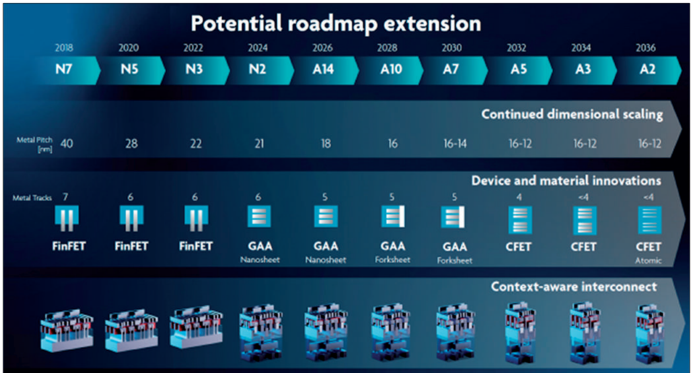
Figure 6. A view on the potential roadmap for continued dimensional scaling, new transistor architectures, new materials introduction, combined with innovative interconnect architectures. (from IMEC “20-year semiconductor roadmap” [49])
