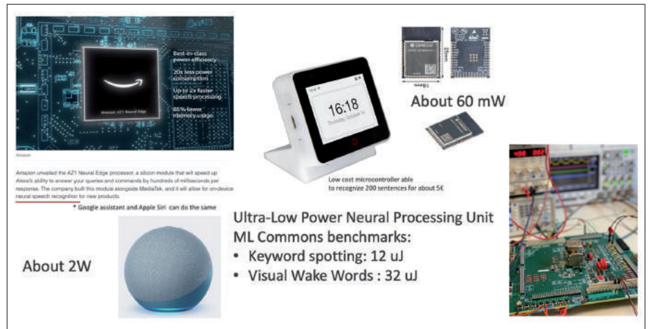
Figure 10: Examples of chips able to carry out (simple) voice recognition locally
