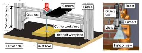
Fig. 2. a): Designed test stand for initial data set generation. b): Demonstrator.
