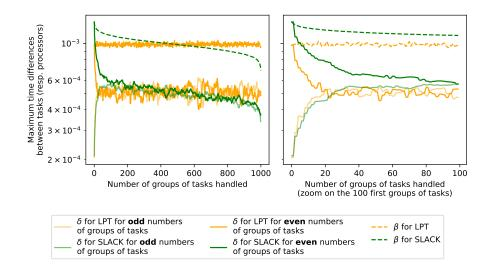
Figure 1: Evolution of  $\delta_j$  and  $\beta_j$  (as defined in Section 3) during the execution of SLACK and LPT with the uniform distribution  $\mathcal{U}[0,1]$  for the tasks. Each execution is done with m=100 processors and  $n=100\,000$  tasks. The right graph is a zoomed version of the 100 first values of  $\delta_j$  and  $\beta_j$ . Each point represents the average value of  $\delta_j$  (resp.  $\beta_j$ ) over 30 executions.
