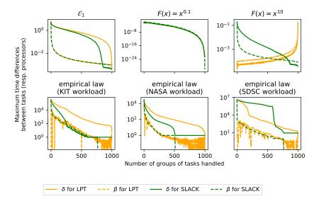
Figure 2: Evolution of  $\delta_j$  and  $\beta_j$  (as defined in Section 3) during the execution of SLACK and LPT with various probability distributions for the tasks. Each execution is done with m=100 processors and  $n=100\,000$  tasks. Each point represents the average value of  $\delta_j$  (resp.  $\beta_j$ ) over 30 executions.
