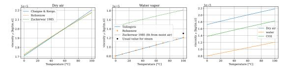
Figure 21: Viscosity from Chaigne and Kergomard, 2016, Rohsenow et al., 1998 and Zuckerwar and Meredith, 1985. If no indications it comes from Rohsenow et al., 1998.
