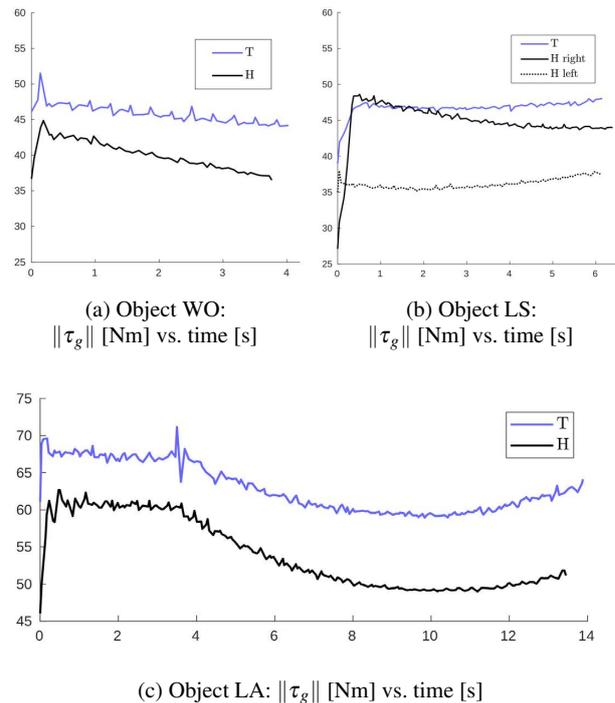
Fig. 10: Time [s] vs. norm of the joint torques  $\|\tau_g\|$  [Nm] during the post-grasp trajectory for T and H control mode and three objects: 10a WO (corresponding with 8a and 8b), 10b LS (corresponding with 8c and 8d), 10c and LA (corresponding with 8e and 8f)
