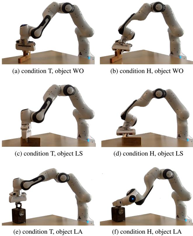
Fig. 8: Grasp poses teleoperated in T (fully teleoperated) and H (haptic-guided shared control teleoperated) mode of control system: **8a**, **8c** and **8e** grasp poses for WO, LS, and LA chosen by the user in T control mode; **8b**, **8d** and **8f** grasp poses for WO, LS, and LA chosen by the user in H control mode
