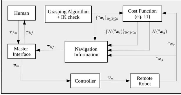
Fig. 4: Block diagram summarising the shared control framework. A set of feasible grasps  $\{{}^o x_i\}$  is generated by a grasping algorithm. Then, we calculate the torque cost function  $H({}^o x_i)$  at each of these poses to design the visuo-haptic feedback  $\tau_{hf}$  to guide the human user. Finally, the operator controls the remote robot in velocity using the grounded haptic interface
