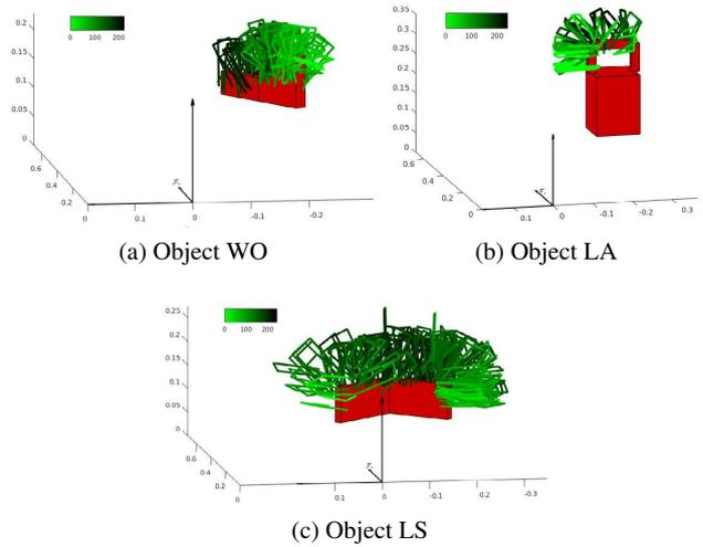
Fig. 6: Feasible grasps and TOTE cost  $H({}^o x_g)$  for the three objects used in our experiments. The grasping candidates are colour-coded according to the corresponding cost value. Lighter green corresponds to a lower cost function
