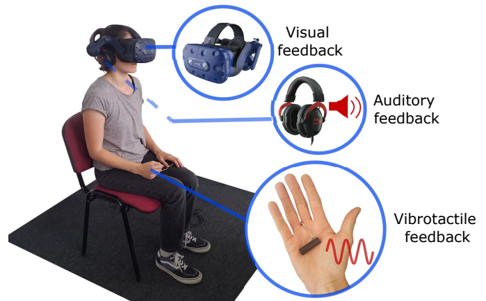
Figure 4: The setup for Experiment I which includes a visual headset, an audio headset and a vibrotactile actuator.
