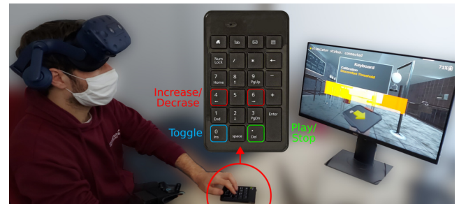
Fig. 9. Desktop-based calibration process using a keyboard. Participant needs to temporarily lift the HMD to look at the monitor.
