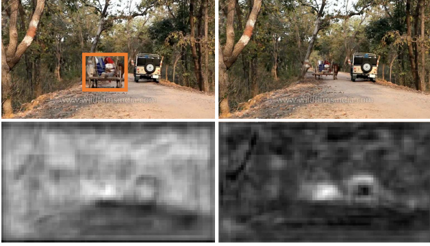
Figure 3: The effect of our proposed discriminative template on an example of a video from GOT-10k dataset [18]. By simply using the center feature of the bounding box around the cart (top left), the resulting attention map (bottom left) for the test frame (top right) is not focused on the object. In contrast, our discriminative template (bottom right) results in a much better attention map.
