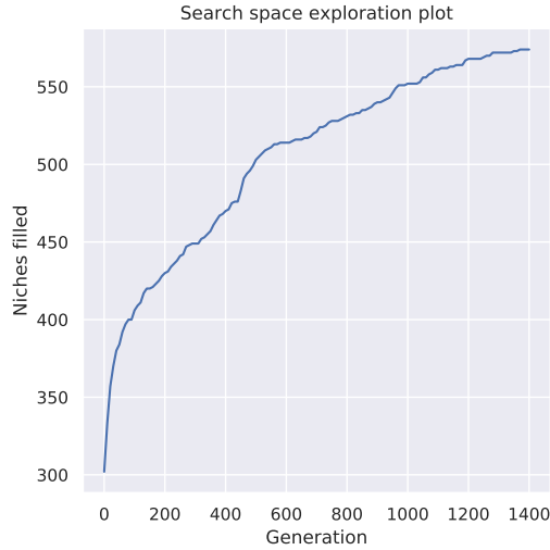
Fig. 3: Exploration progress, showing the number of niches filled against the number of generations. Generation 0 happens after the initialisation phase of the MAP-Elites algorithm, in which seed objects are randomly generated for the evolutionary exploration. Each generation explores 128 new object samples. The curve represents two weeks of continuous sequential computation on a server computer.
