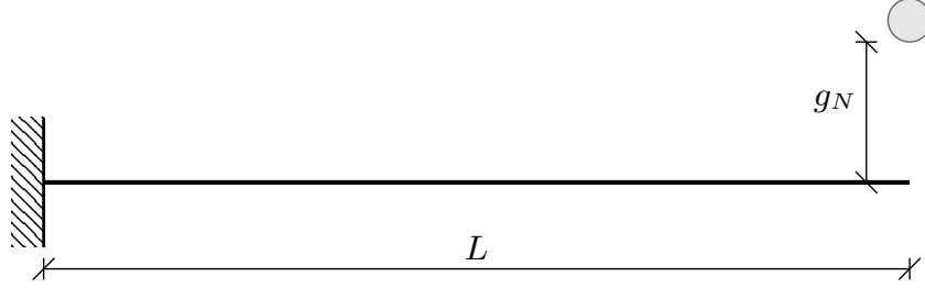
Figure 16: Example 2: impacted cantilever beam.
