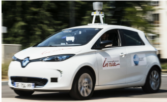
Fig. 6. Experimental Platform: Renault Zoe car equipped with Velodyne HDL64, 4 Ibeo Lux LiDARs, cameras, Xsens GPS and IMU.
