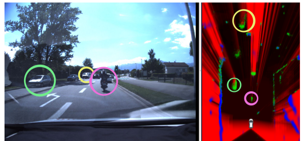
Fig. 10. Camera, and filtered state grid showing static occupancy (blue), dynamic occupancy (green) empty space (black) and undefined areas (red).
