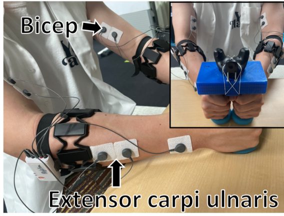
Fig. 4. The sEMG sensor electrodes were attached to the user's ECUs and biceps. Participants held the dumbbells with both hands. The tracker was mounted on the dumbbell pair to track the user's arm movement.
