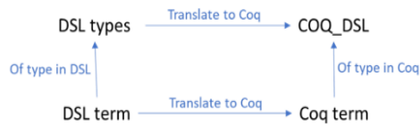
Fig. 2. Commutativity diagram between DSL and COQ terms
