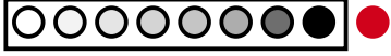
Fig. 2: The nearest neighbors have different weights that depend on their position (proportional to their age) in the window. The white point represents the oldest instance in the window with the lowest weight, while the black one represent the most recent with the highest weight.
