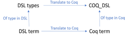
Fig. 2. Commutativity diagram between DSL and COQ terms
