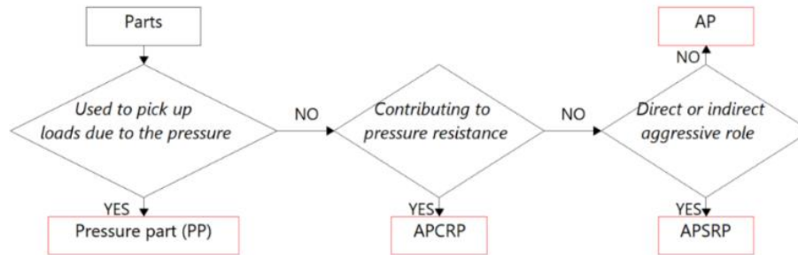
Fig. 10. Component classification logic
