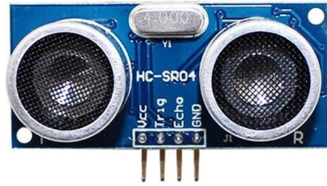
Fig. 2. The HC-SR04 is ubiquitous in robotic platforms to measure distance to obstacles. It is very easy to find and very cheap. RRDV re-uses it to detect encounters between robots. Note that the CWL-1601 is an equivalent sensor, operating at 3.3 V.
