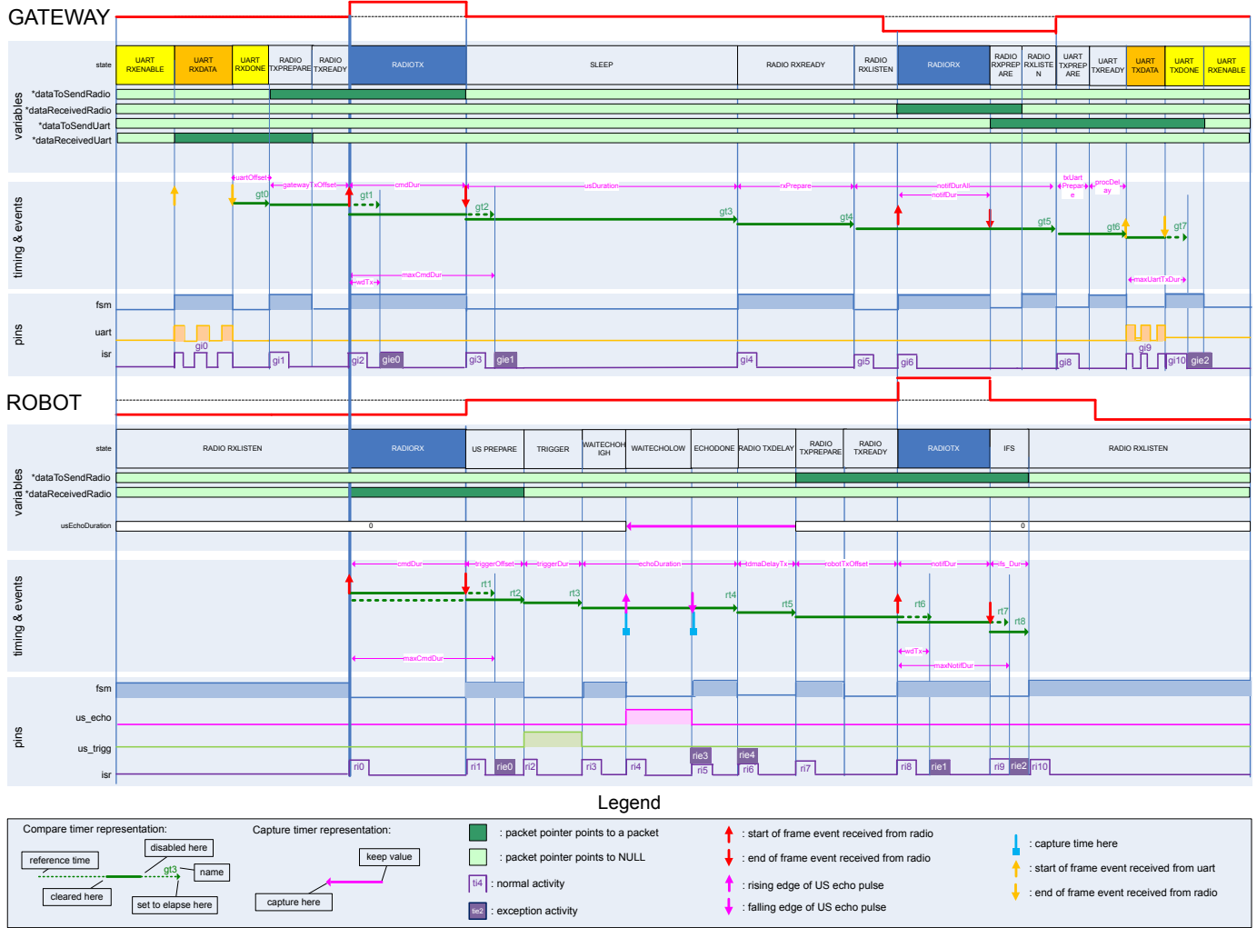
Fig. 5. Chronogram of the RRDV state machine representing the activity of a gateway and mobile robot. The figure shows their radio activity (red line), events and timers, value of the global variables and the state of the debug pins.
