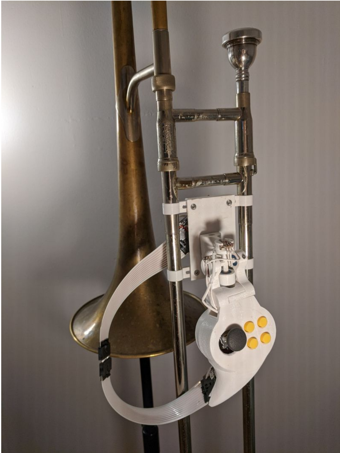
Image 2 The first version of the yoke controller.
