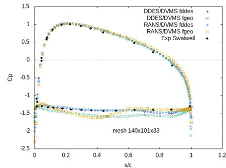
Figure 3: Mean pressure coefficient over the airfoil surface.
