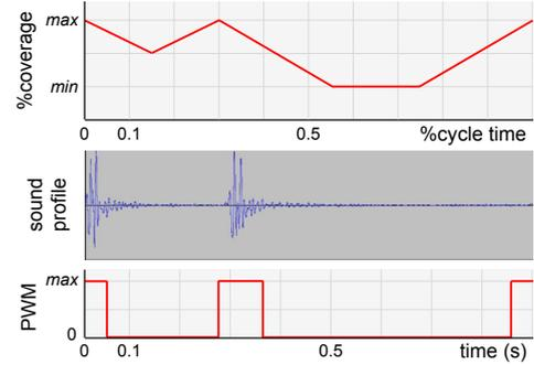
Fig. 3. Variation of Tunneling coverage, Sound profile, and PWM during a cardiac cycle
