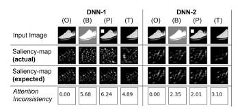
Fig. 2. Differences in changes in saliency-maps for two DNNs. Each saliency-map of DNN-1 above is more collapsed than DNN-2's: where columns (O), (B), (P), and (T) denote original (i.e., without perturbations), brightness change, patch, and translation, respectively.
