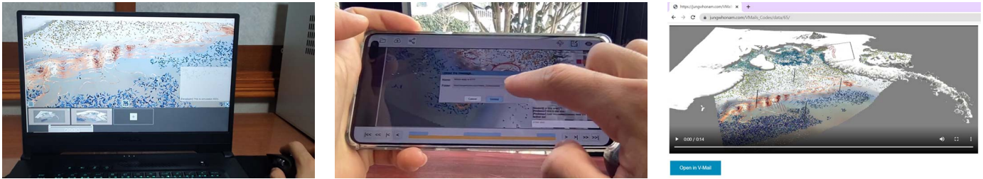
Fig. 1. Three working platforms that demonstrate different storytelling fidelities of V-Mail for analyzing Antarctic ice-sheet data: (right) anyone with a video player can at least passively view the story, including annotations made by others; (left) in the highest-fidelity case, the story unlocks data on a V-Mail server than can be loaded via a plugin for desktop-based visualization applications, where users can explore and annotate the 3D data more deeply; (middle) the mobile client works as a custom video player with mechanisms for interactively viewing the story and adding annotations.
