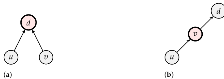
Figure 12. One transceiver cannot be involved in multiple communications within the same timeslot. (a) Simultaneous transmission to the same parent. (b) Simultaneous reception and transmission.
